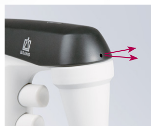
Direct outlet of sample vapors
