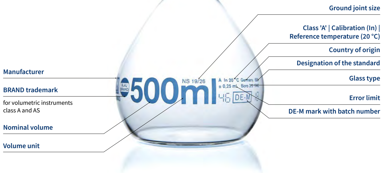
BLAUBRAND® volumetric flask, class A
