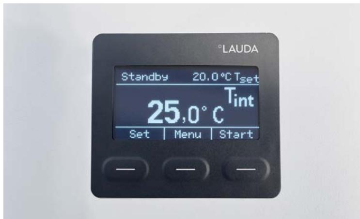
Simple three-button controls with OLED display
