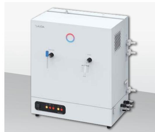
Equipped for any application: Puridest PD 4 D for the direct distillate extraction of mono- or bi-distillate
