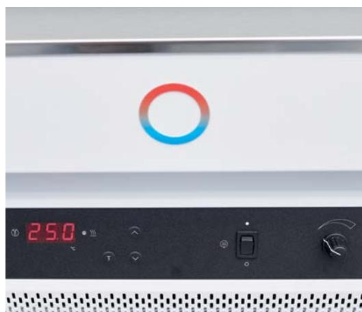
Operation left: Temperature adjustment with LED display,
