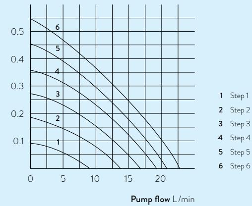
**PUMP CHARACTERISTIC** for PB and PBC, Water
