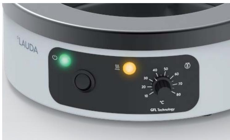
Adjustable bath temperature with heating activity display
