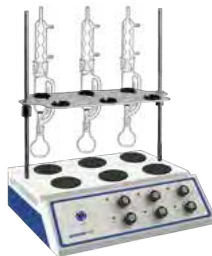
Parallel reaction for Soxhlet extraction
