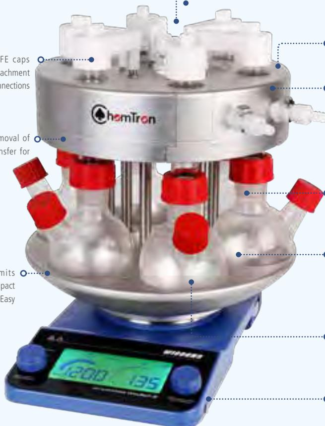
Central inlet/outlet for vacuum and gas, combined with a radial gas distribution system and gas-tight PTFE caps, allow reactions under an inert atmosphere
