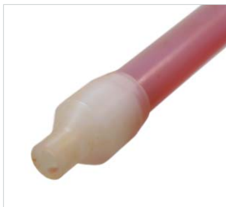
Sampler Tip Seal arrangement prevents sample from dripping
