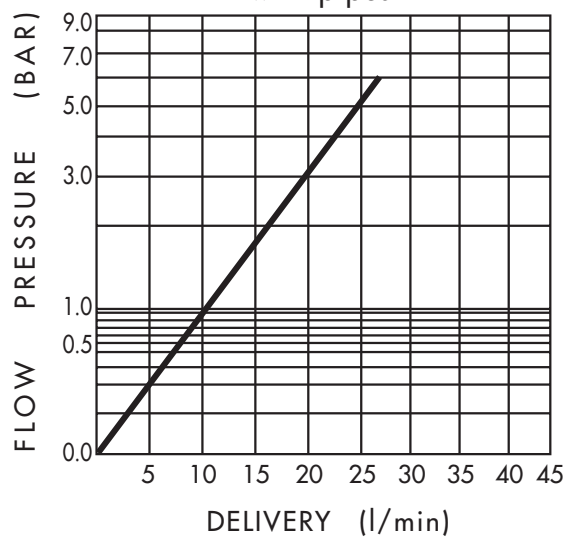
1000/130 Fume cupboard valve with pipes
