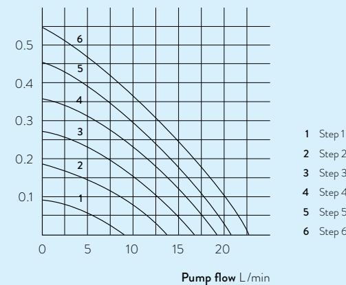
**PUMP CHARACTERISTIC** for PB and PBC, Water
