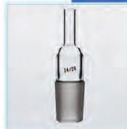
温度计套管 Adapter for thermometer
