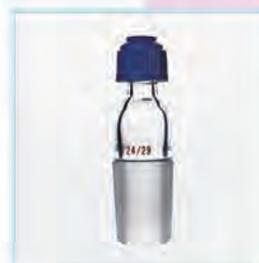
密封搅拌器套管 Adapter for stirrer
