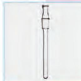
螺口温度计套管 Adapter,inlet for thermometer
