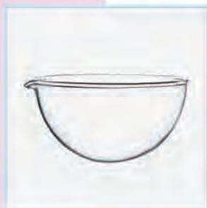
石英圆底蒸发皿 Quartz evaporating dish,round bottom
