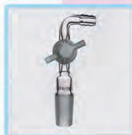
具T型玻璃节门三通接头 Adapter,T-bore glass stopcock
