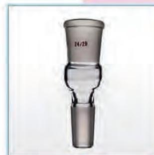
球磨口与标准塞互换接头 Adapter,with ball socket
